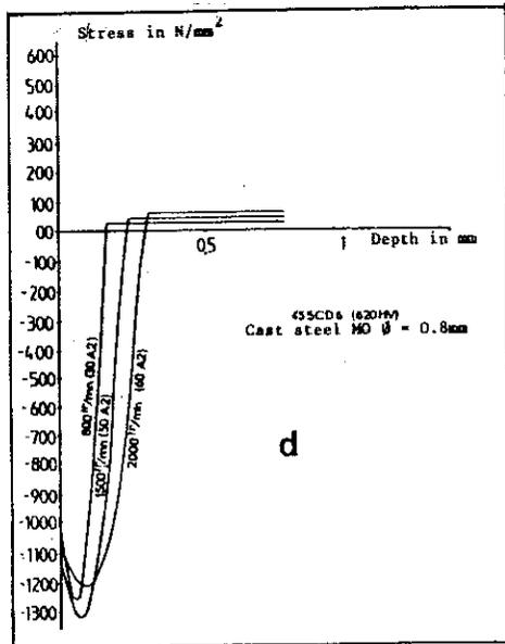
Fig. 9d. The effect of the Almen intensity and the shot velocity on the distribution of residual stresses
