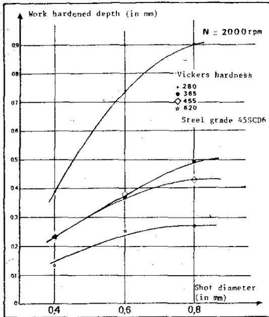
Fig.4. The effect of the shot diameter on the depth of the work hardened strata
