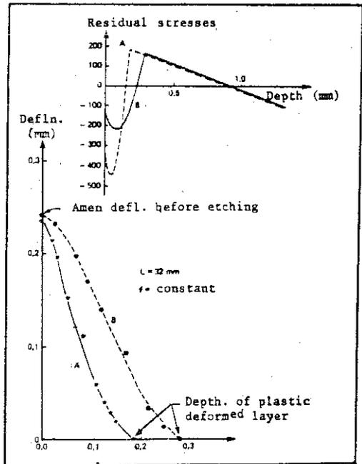
Fig 1b. Curves of deflection and residual stress obtained on two Almen test pieces with the same initial deflection.
