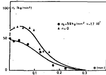
Fig. 13. The distribution of residual caused by shot-peening before and after the part has been subjected to fatigue
