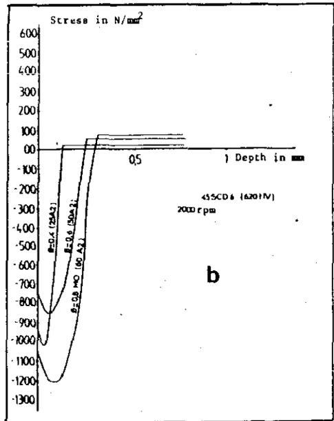
**Fig. 11b. The effect of the shot diameter on the residual stress -distribution**
