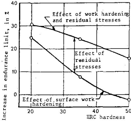
Fig.12. The respective effect of residual stresses and work hardening on the increase in the fatigue limit of the shot peened materials
