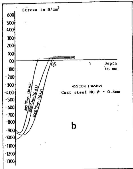
Fig. 9b. The effect of the Almen intensity and the shot velocity on the distribution of residual stresses
